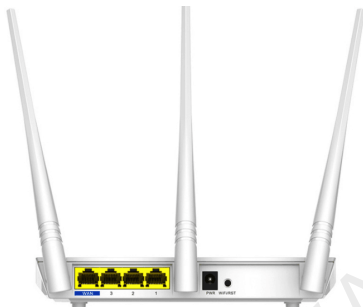
Figure 6-2 Ports of wireless router
