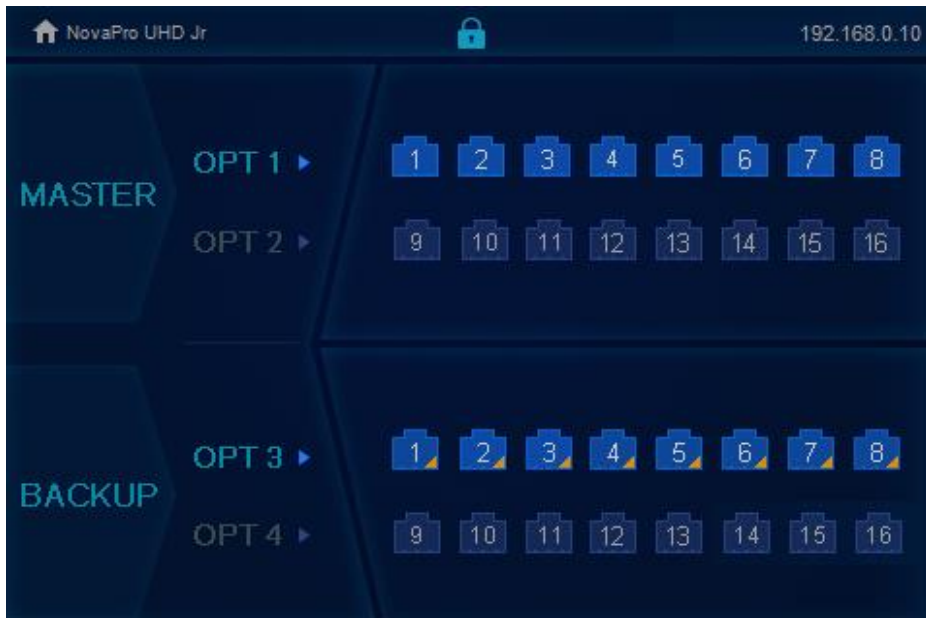
Figure 4-3 Optical fiber port statuses – Hot backup
