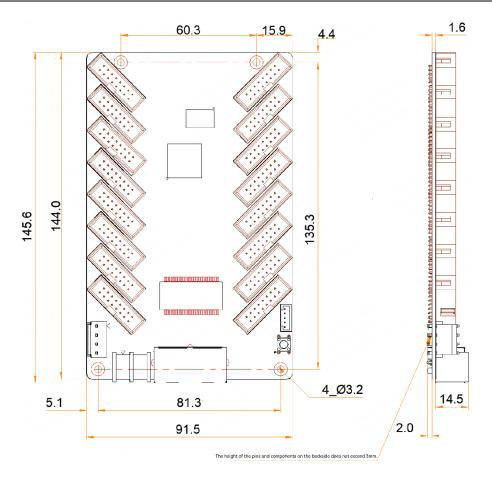
Tolerance: ±0.3 Unit: mm
