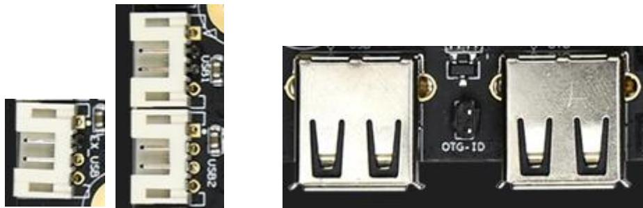
The board has 2 USB standard interfaces and 3 USB pins, one of which is shared with the 4G module.
