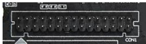
General LVDS interface definition, support single/dual, 6/8/10-bit 1080P LVDS screen. The screen voltage can be selected through the jumper cap, and the screen power supply can be selected to support 3.3V/5V/12V.
