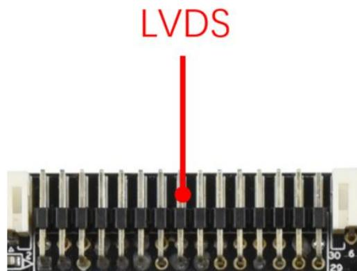
General LVDS interface definition, support single/dual, 6/8/10 bit 1080P LVDS screen. The screen voltage can be selected through the bridle-wire cap, and can choose to support 3.3V/5V/12V screen power supply.
