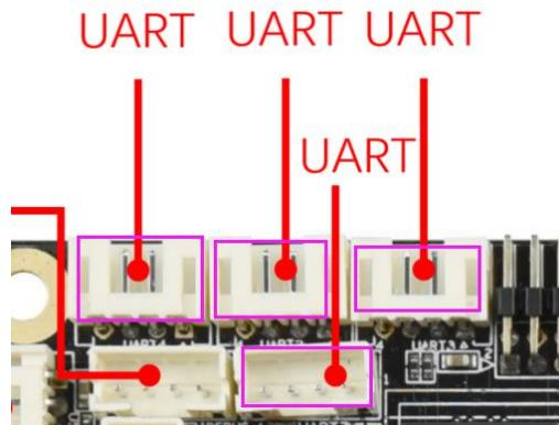
The motherboard leads to two sets of common UART serial ports, which can support common UART serial devices on the market.
