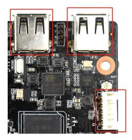
The motherboard has 2 USB standard interfaces and 1 USB pin
