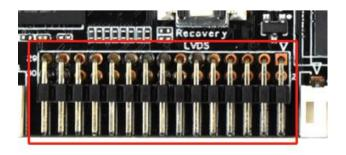
General LVDS interface definition, support single/dual, 6/8/10 bit 1080P LVDS screen. The screen voltage can be selected through the bridle-wire cap, and can choose to support 3.3V/5V/12V screen power supply.
