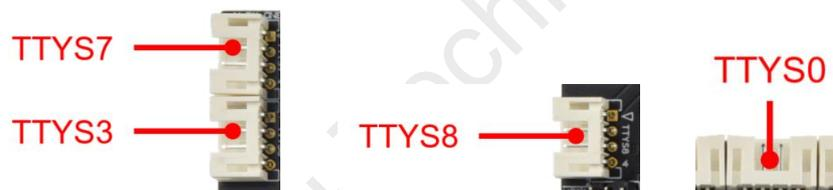
1 set of ordinary two-wire serial ports, which can support common serial devices on the market. The level of the serial ports is 0V to 3.3V. If the level of the connected serial port is higher than 3.3V, there must be an isolation circuit or a level conversion circuit, otherwise the main control and equipment will be burned out.
