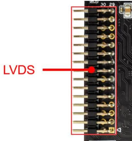
General LVDS interface definition, support single/dual, 6/8/10 bit 1080P LVDS screen. The screen voltage can be selected through the jumper cap, and can choose to support 3.3V/5V/12V screen power supply.
