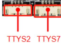
The board leads to two sets of ordinary UART serial ports, which can support common UART serial port devices on the market.
