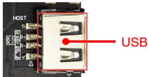
The board has 1 USB standard interface and 1 Mini USB interface
