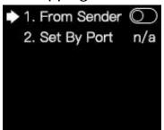
In the submenu, press the knob/OK to set the sender as the connection source. Then select **Set by Port** to enter the submenu, in which you can choose the Ethernet port from 1 to 12 that needs setting mapping, and set the offset values of X and Y, and the width, height, row number, column number and link type of the corresponding cabinets. Finally select **Save** to save the mapping.
