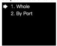
Output shift contains two selections: Whole and By Port. On the submenu of Whole, you can rotate the knob to set the row starting point (X) and the column starting point (Y) of the whole image and then save the setting; on the submenu of By Port, you can respectively set the row starting point (X) and the column starting point (Y) of the image of the 12 Ethernet ports, and then save the setting.
